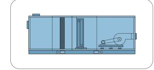
Mixing section + pre-filter section + coil section + heating section + fan section
