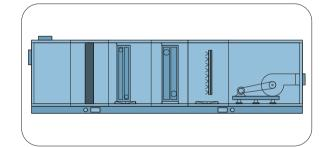
Mixing section + pre-filter section + coil section + heating section + humidification section + fan section + blank section + medium filter section + air discharge section
