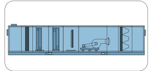
Mixing section + pre-filter section + coil section+ heating section + humidification section + fan section
