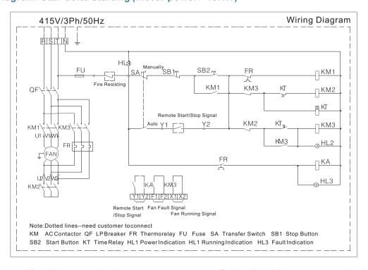
The user lines are directly connected to the motor connector post. During the wiring process; overload, short circuit and overheating protections must be installed
