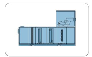
Mixing section + pre-filter section + coil section + heating section + humidification section + fan section + Blank section + medium filter + Air discharge section
