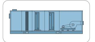
Mixing section + pre-filter section + coil section + heating section + humidification section + fan section
