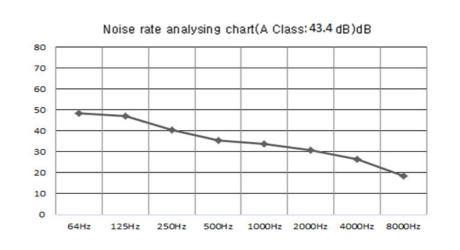
Note:1m from source with 1m insulated duct and fully reflective surface surrounding unit.
